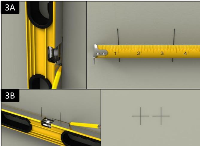
• As illustrated in 3A - Use a level to determine position of right spacer and mark a vertical line. Measure precisely 2 3/8" from this line to locate the position of left spacer.
