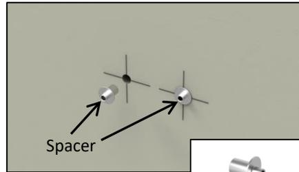
• Insert both left and right spacers into drilled holes. Press in firmly so that flange mounts flush with gypsum wallboard (drywall) material.
