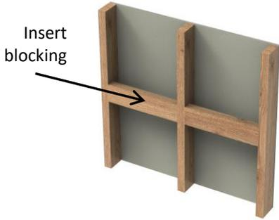
• Insert no less than 2" x 4" wood blocking or locate in vertical stud.
